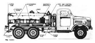
Figure 6-66. Decontamination equipment. The ARS-12U truck-mounted decontamination system (above) consists of a large tank on a truck chassis with hoses, brushes, and special-purpose nozzles. One filling of the 680-gallon tank can decontaminate about 12 tanks. The DDA-53 (below) consists of two steam chambers and a boiler, and is used to decontaminate clothing, small arms, and light equipment.
